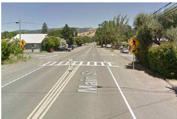
Figure 177: Main Street in Old Hopland, looking north towards crossing to be replaced with high visibility crosswalk (Source: Google Street View)
