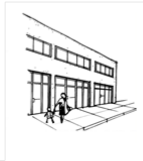
Without architectural variations buildings appear flat, larger, and "box like"
