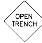
4 (C27 CA) Black on Orange 24" X 24" (or 36" x 36" Optional) 4" Lettering (D Series)
